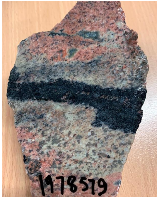
Photograph of sample 1978579. The coarse-grained dark alteration cuts the pre-existing granitic fabric and is also associated with sericitisation of the feldspar.
